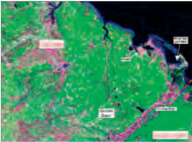
RUVUMA - RGB satellite image of the Tanzanian coastal portion of the Ruvuma Basin – Aminex’s licence covers most of the area in the image. Such images are extremely helpful to the exploration process, from using landforms such as rivers and outcrop geology to predict the deeper underlying structural geology, to assisting with determining logistics for efficient seismic acquisition.
